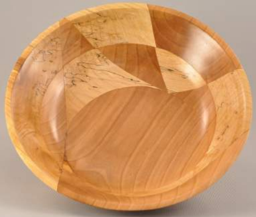
Jerry Holbrook Cherry & Spalted Maple Segmented Bowl Salad Bowl Finish Used bandsaw to cut 2 stacked pieces then glued
